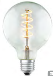
TLB-8007-04CL LED SPIRAL GLOBE G80 E27 2200K 4 W=15 W | 180 lm 25.000 hours CRI 80 8 CM 12.3 CM CERTIFICATE: DEKRA
